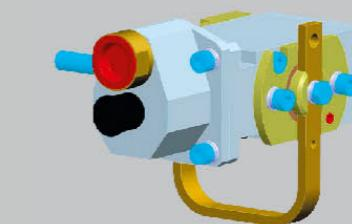
Emergency release valve 370 (КС 370) is intended to provide automatic emergency discharging of the brake pipe when the train passes the restrictive track signal, as well as when exceeding the prescribed train speed at track sections equipped with inertial busbars.
