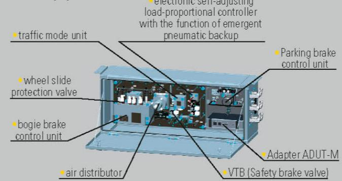
The brake equipment unit 072 (БТО 072) is used on subway cars with design speed of 90 km/h that are operated in the tunnels on the existing underground lines and in the open areas of the railroad featuring with the bottom location of contact of the contact rail.
